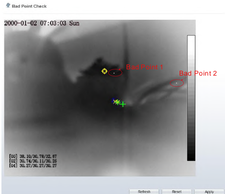
Figure 4-16 Bad Point Check
