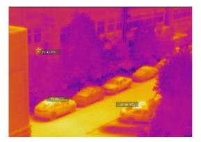
When selecting point analysis, you can move the mouse and click Add Temperature Points, you can add up to 20 temperature points. If an individual point needs to be edited, select it, then right-click the mouse, select Edit Option to adjust local parameters (different from global parameters), delete or set as reference temperature.
