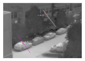
When selecting line analysis, you can move the mouse to click and drag where you want to add the temperature measuring points. You can add up to 20 temperature lines. By default, the point of maximum temperature on this line segment (small red arrow up) is displayed.
