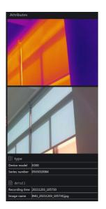
When selecting images in the thumbnail column, the information contained in this image such as the infrared image, visible light image, shooting time and the serial number of the camera will be displayed on the right side
