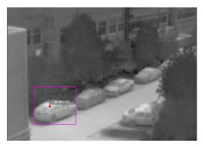
When selecting area analysis, you can move the mouse to click and drag where you want to add the temperature measurement area, and you can add up to 20 temperature measurement areas. The default display is the point of maximum temperature in this area (the little red arrow up).
